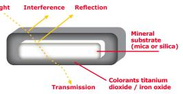
Schematic representation of a Candurin® platelet: The arrows depict light which can be seen as being reflected, refracted and transmitted simultaneously to produce the play of colors known as pearlescence.
